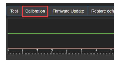
2 At the test page. Click the following button for calibration. Move Z axis full range for calibration;
