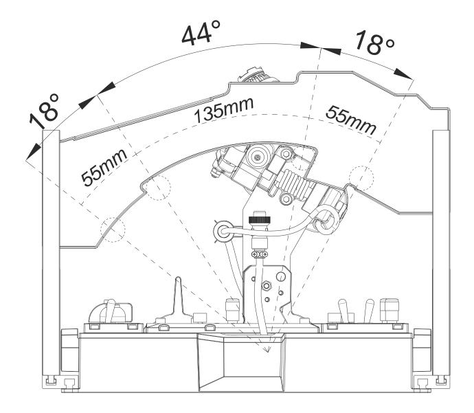
Total movement angle 80 (Idle to stop 18, normal thrust 44, afterburner 18)
